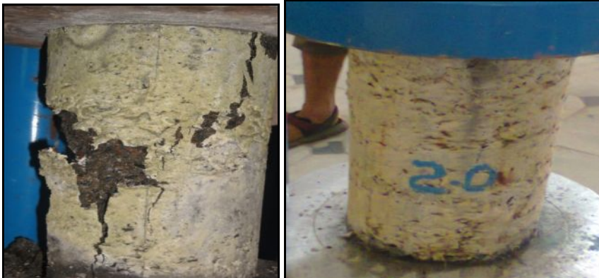
Figure 1. Failure pattern due to compression test
