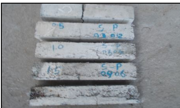
Figure 3. Failure pattern of HSC, and HYFRC specimens due to Flexural test
