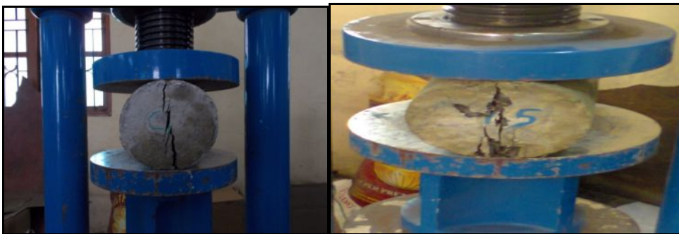
Figure 2. Failure pattern due to Splitting tensile test
