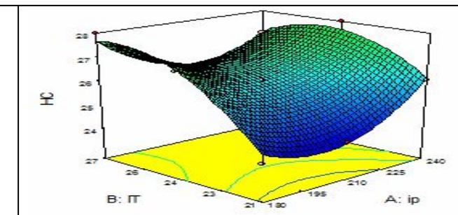
**Fig – 4 (a) 3D Surface Plot Variation of HC between Injection Pressure and Injection Timing**
