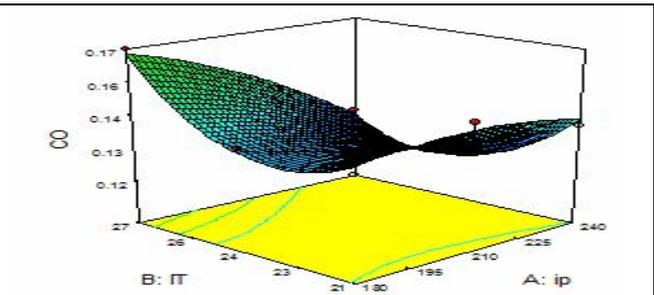
**Fig – 2(a) 3D Surface Plot Variation of CO between Injection Pressure and Injection Timing**
