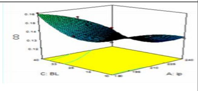
**FFig – 2(c) 3D Surface Plot Variation of CO between Injection Pressure and Injection Timing**
