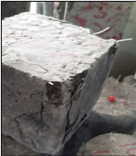
Figure 4 Failure of cube Specimen
