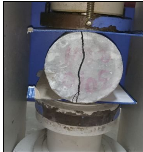
Figure 5 Failure of Cylindrical specimen
