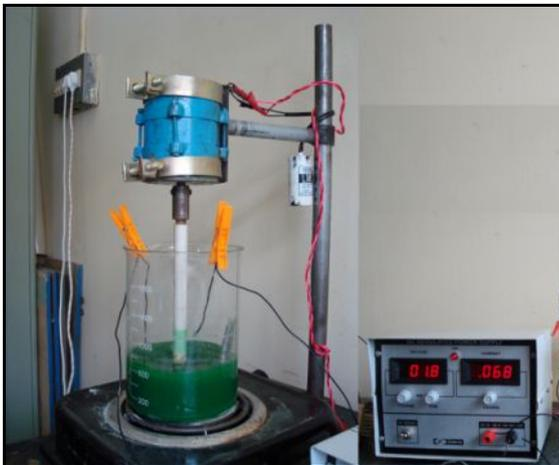
**Fig .1. Electroplating Experimental Setup**
