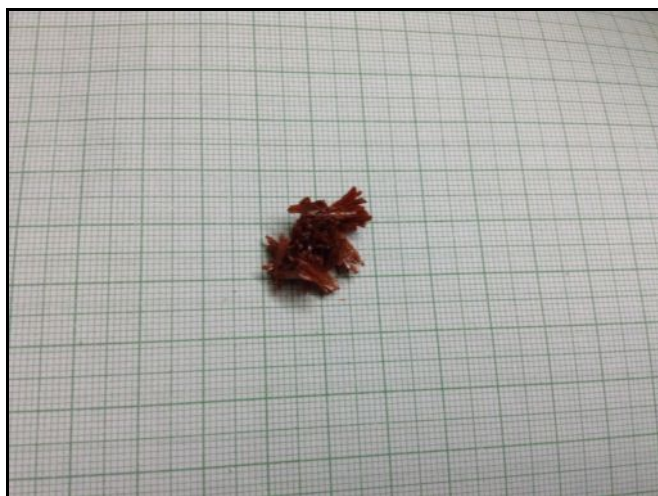
Fig.(1) The grown single crystal of 4Cl 2 NA.
