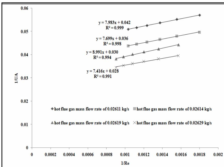
Figure 7: Wilson plot analysis of cast iron porous tube
