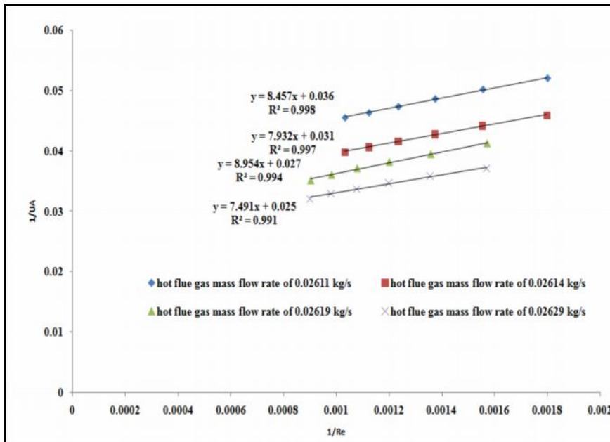
Figure 6: Wilson plot analysis of Mild Steel porous tube
