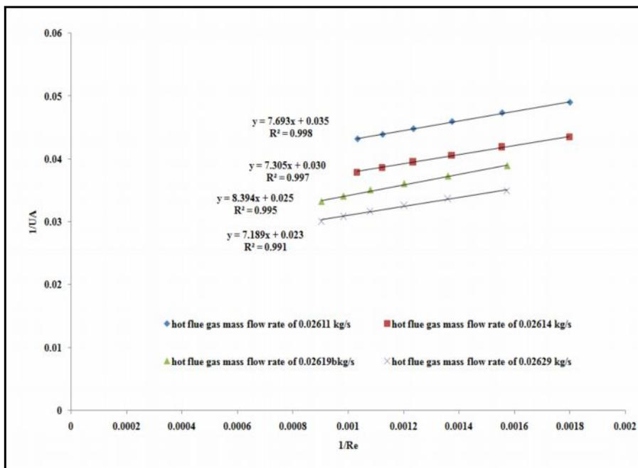
Figure 5: Wilson plot analysis of Copper porous tube
