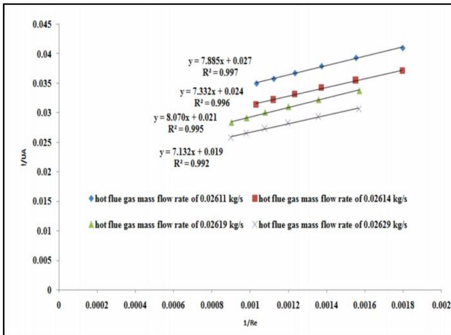
Figure 4: Wilson plot analysis of Aluminum porous tube
