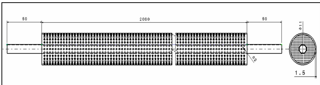
**Figure 1: Geometric view of inner porous tube**
