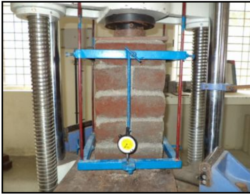
Figure 3 Test set-up of brick masonry prism
