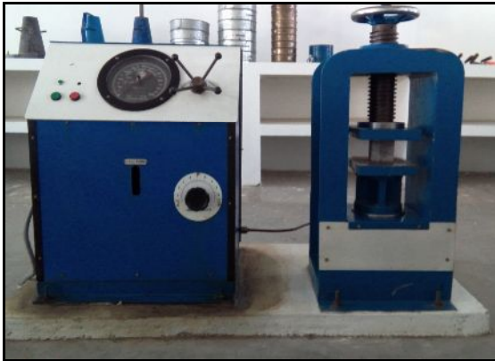
Figure 2 Test set-up of cement mortar cube
