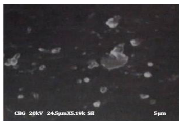
Fig.9 SEM image of SPSEBS-SiO 2 -SO 3 H 7.5% composite membrane
