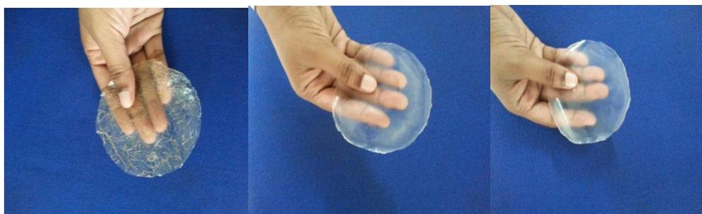
**Figure 3.Macroscopic visual images of starch biocomposites with 6% loading of A. Alkali hydrolysed, B.Bleached and C. Cellulose nanocrystals.**
