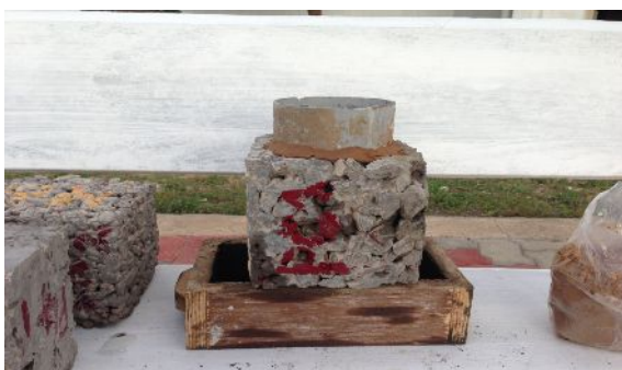
Fig 2 Infiltration test using single ring infiltrometer
