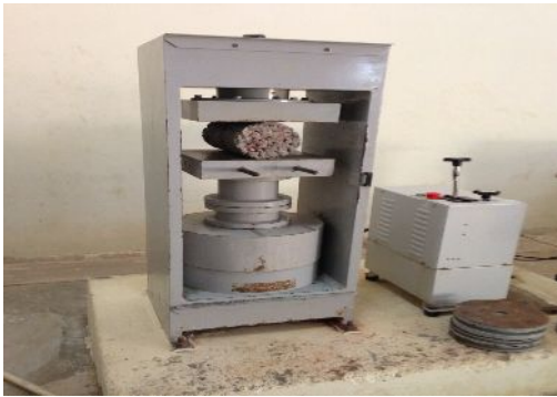
Fig 1(b) Cylinder under split tensile test
