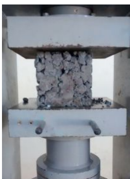
Fig 1(a) Cube under compression test
