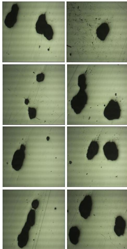
Figure 3 Corroded Specimens of Conventional processing
