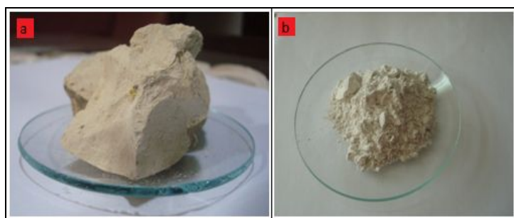
Fig.3. Sample a) Natural bentonite from North Aceh and b) MMT isolation results
