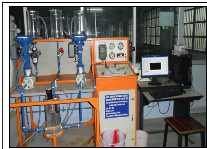
Figure 1. Real Time Experimental Setup of pH Neutralization
