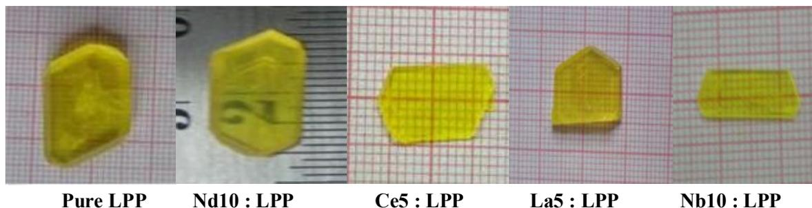
Figure 1. As grown pure LPP and doped LPP crystals
