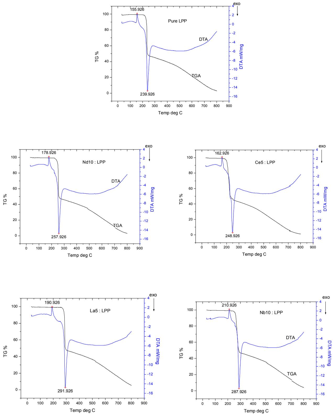
**Figure 3. TG-DTA graph for pure and doped LPP samples**
