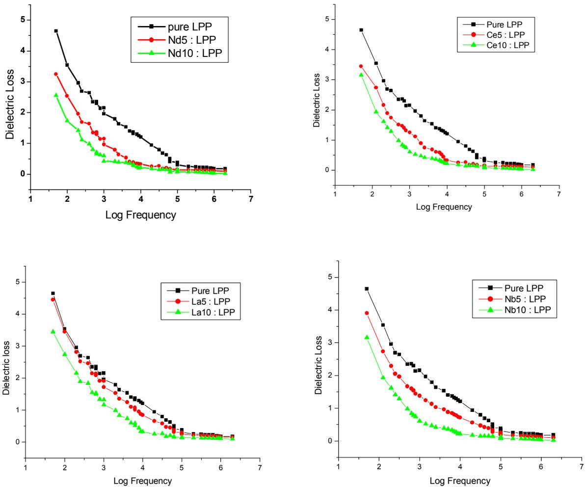
Figure 2 (b). Dielectric Loss vs. Log frequency for pure and doped LPP crystals
