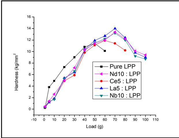
**Figure 5. Microhardness measurement for pure and doped LPP crystals**
