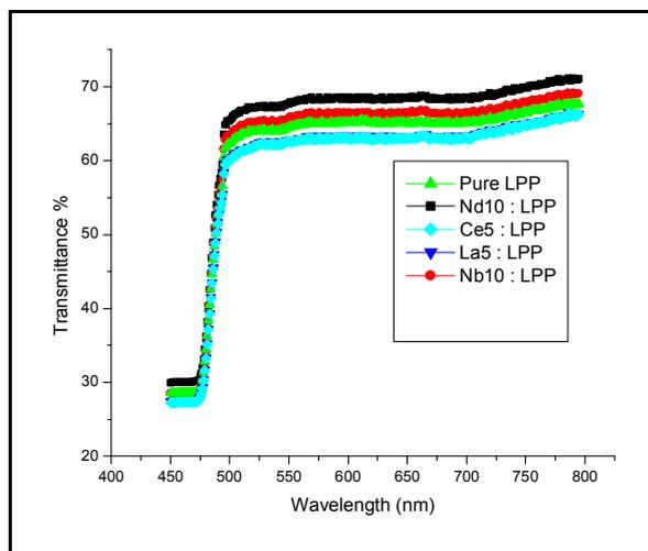
**Figure 4. Optical transmission for pure and doped LPP crystals**
