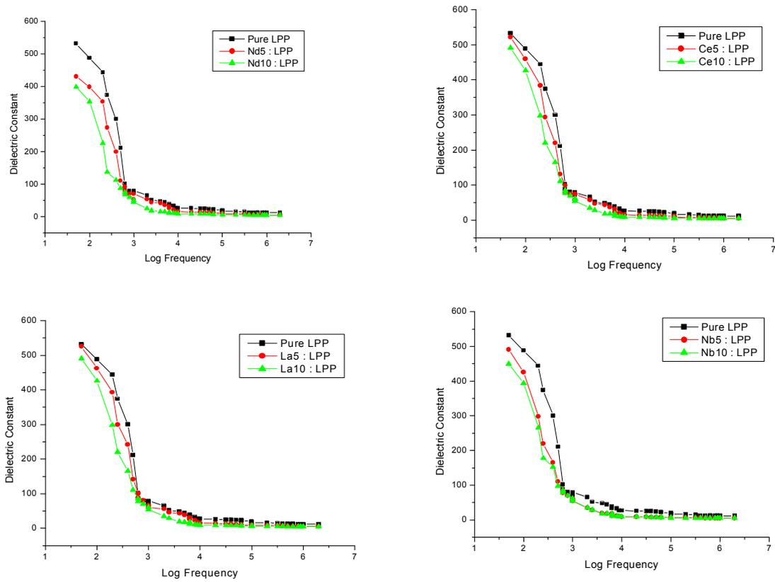
Figure 2 (a). Dielectric Constant vs. Log frequency for pure and doped LPP crystals
