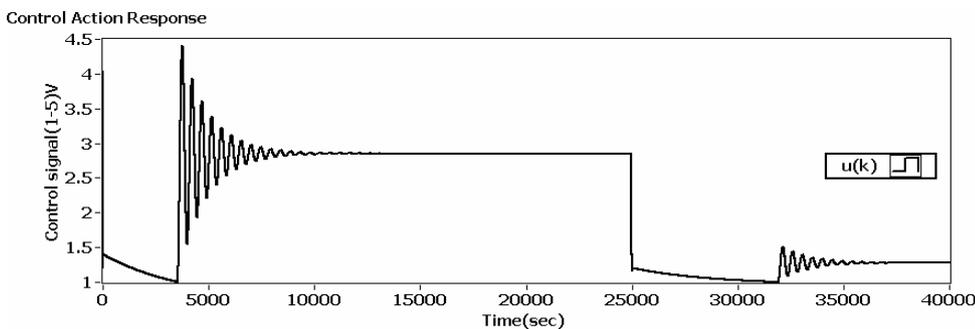
**Figure 10. Control Input – State Estimation based MPC**
