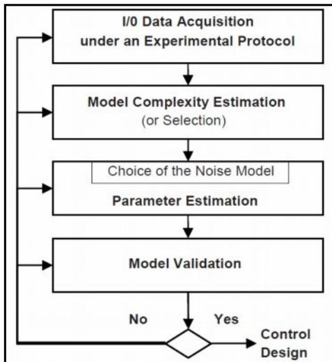
**Figure 1. Flow diagram of System Identification**
