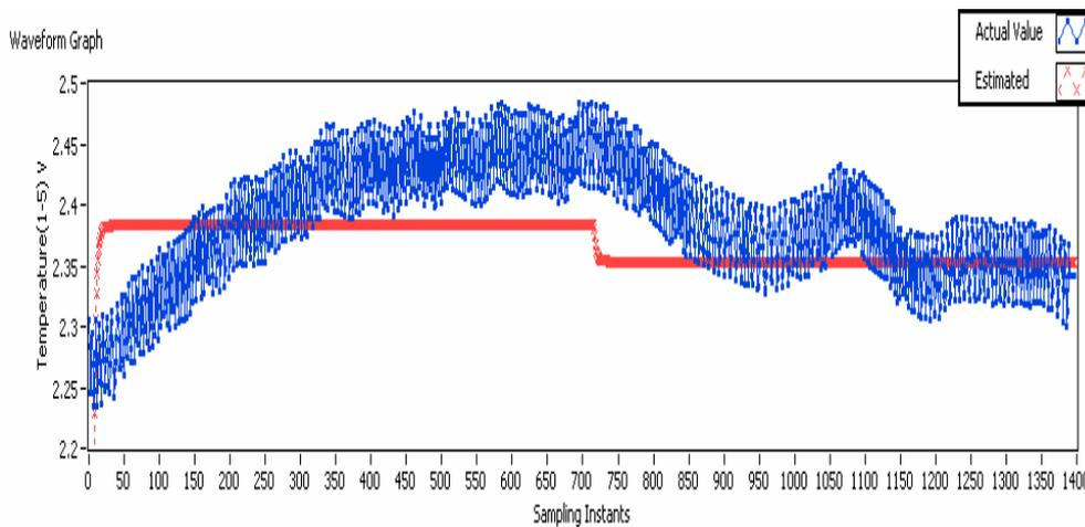
**Figure 4. Comparison of Open loop response of Actual plant and Identified Model**
