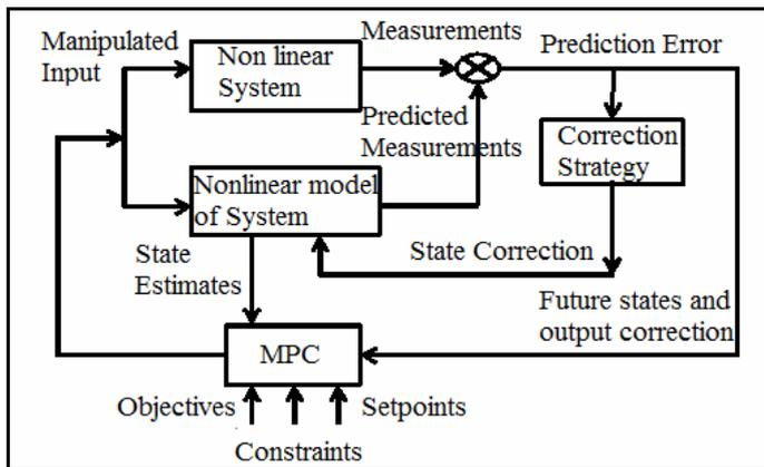
**Figure 6. Block Diagram of State Estimation (Virtual Feedback) Based MPC**
