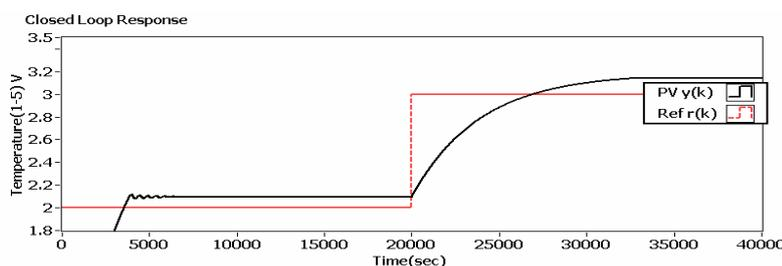
Figure 7. Closed Loop Response - Conventional MPC
