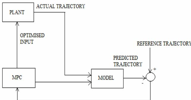
**Figure 5. Block Diagram of MPC controller**
