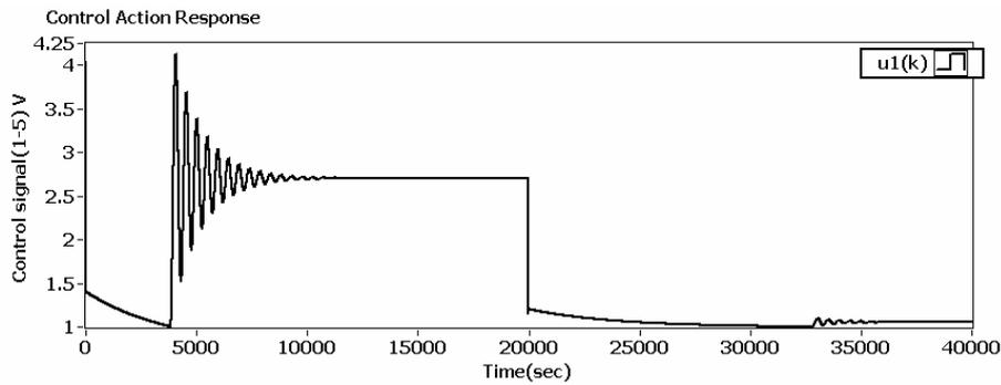
**Figure 8. Control Input – Conventional MPC**
