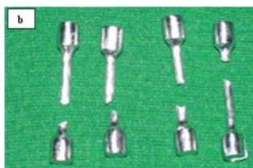
**Fig. 4b Fractured tensile test specimens of Co-Cr alloy after tensile testing**
