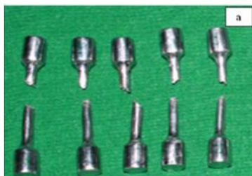
**Fig. 4a Fractured tensile test specimens of Ni-Cr alloy after tensile testing**
