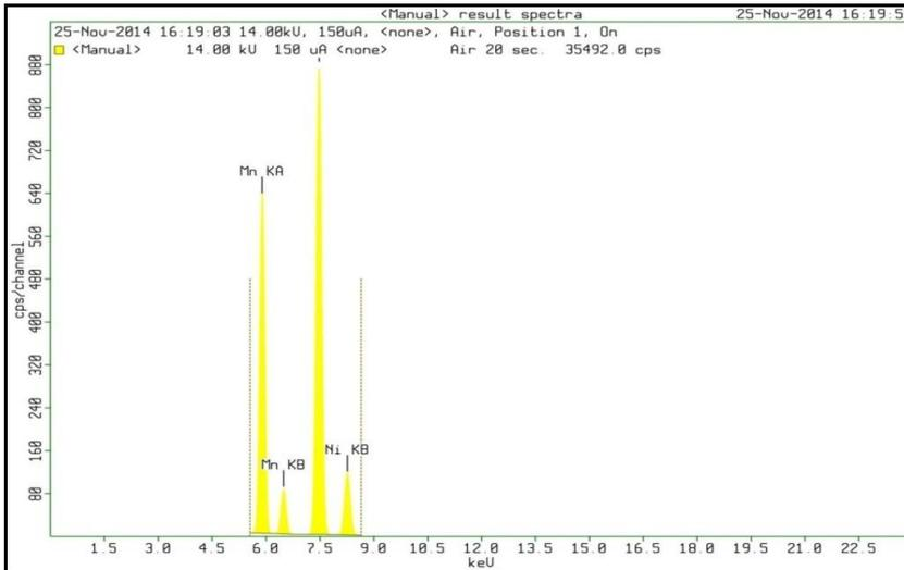
**Fig.5b XRF Analysis for NiO/MnO nanocomposites.**
