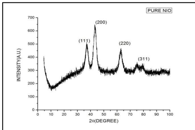
**Fig.2 XRD pattern of NiO nanoparticles**
