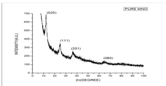
Fig.1 XRD pattern of Pure MnO nanoparticles
