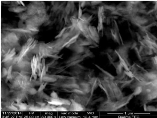
**Fig.4(a) SEM image of NiO/MnO nanocomposite with 1micrometer**
