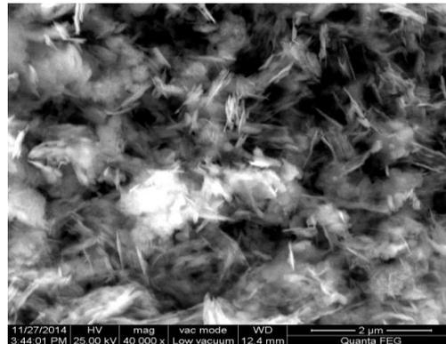
**Fig (4b) SEM image of NiO/MnO nanocomposite with 2 micrometer**
