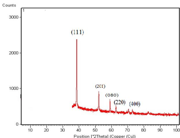
**Fig.3 XRD pattern of NiO/MnO nanocomposites**
