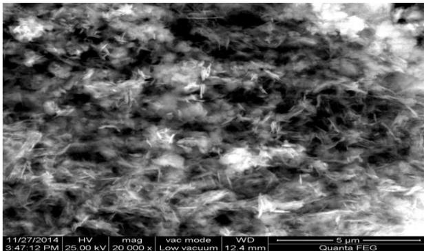
**Fig.4(c) SEM image of NiO/MnO nanocomposite with 5 micrometer**
