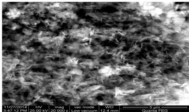
**Fig.4(c) SEM image of NiO/MnO nanocomposite with 5 micrometer**
