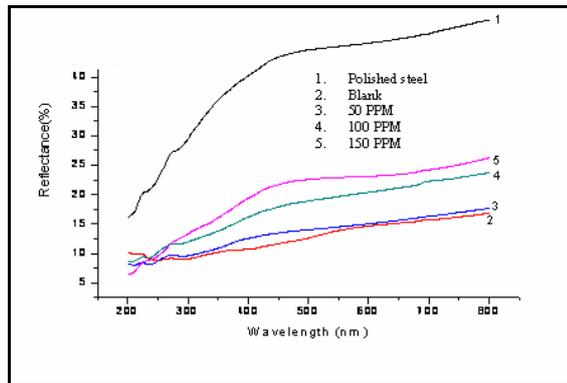
**Figure 2. UV Reflectance curves for reinforcing Steel in simulated concrete pore solution with different concentrations of Mezlocillin.**
