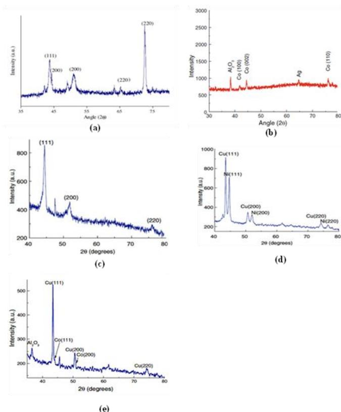
**Figure 1** XRD pattenen of synthesised nanowire (a) Cu nanowires (b) Co nanowires (c) Ni nanowires (d) Cu-Ni nanowires (e) Cu-Co nanowires
