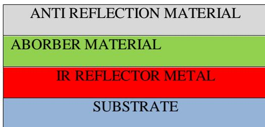
**Figure 2. Schematic diagram of the solar selective absorber coating**
