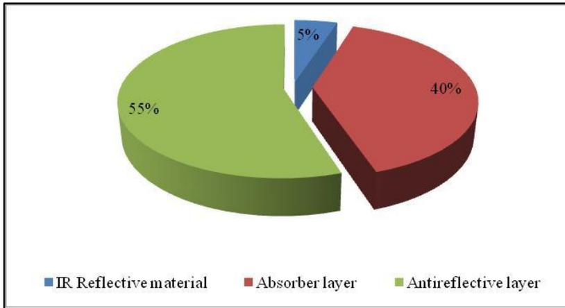
Figure 5 Graph shows the percentile effect of the factors on absorptance
