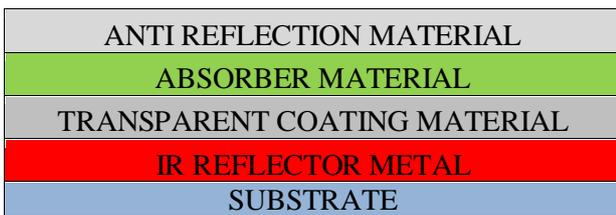
**Fig. 4 Schematic diagram of the solar selective absorber coating**
