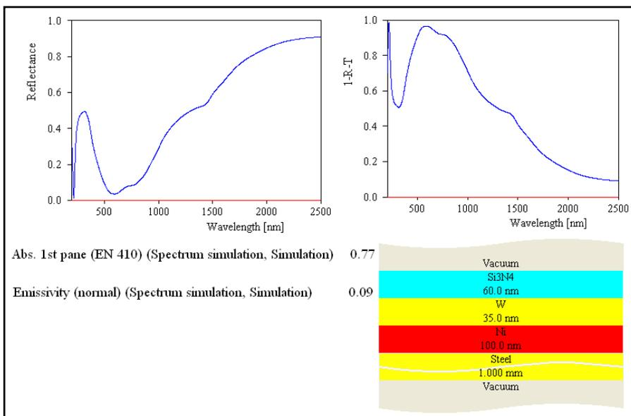
Figure 7 Optimized solar selective multilayer coating
