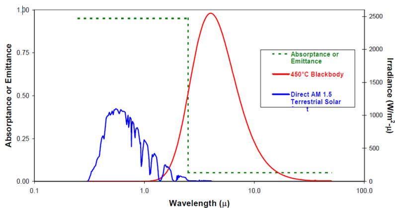
**Figure 1. Spectral performance of an ideal selective solar absorber.** (Courtesy of 6)
