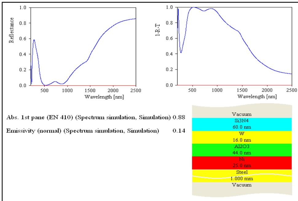
**Figure 8 Effect of introducing dielectric layer in between IR reflector and absorber solar selective multilayer coating**
