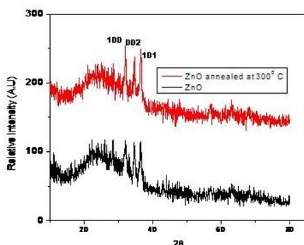
Figure 3 XRD patterns of ZnO as prepared and 300<sup>0</sup> C thin films
