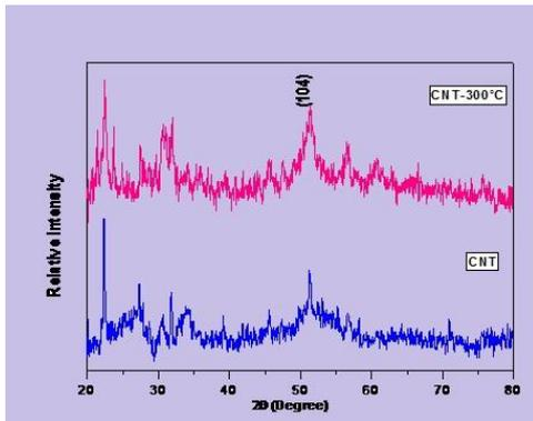
Figure 1 XRD pattern of CNT as prepared and 300<sup>0</sup> C thin films
