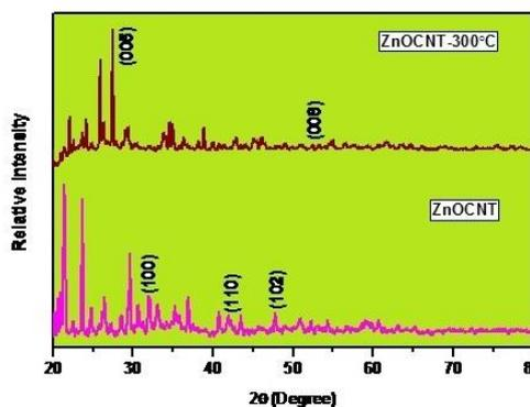
Figure 2 XRD pattern of ZnO-CNT as prepared and 300<sup>0</sup> C thin films
