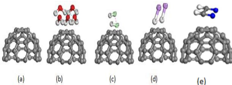
**Fig.2. Highest Occupied Molecular orbital for the following : (a) Carbon nanotube (b) Two water molecules with nanotube (c) Two HCl molecules with nanotube (d) two LiH molecules with nanotube (e) two HCN molecules with nanotube**
