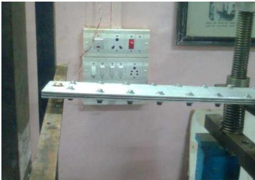
**Fig.2(a). Prepared MR Fluid Sandwiched beam**
