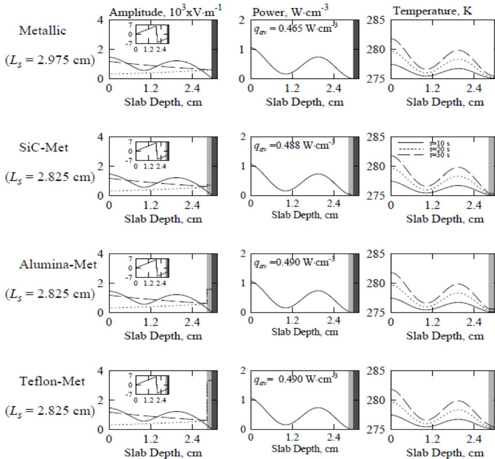
**Figure 4: Spatial Distributions of Amplitudes of Electric Field, Power and Temperature for Blood Samples Placed on Metallic, SiC-Metallic, Alumina-Metallic and Teflon-Metallic Supports During R2 Mode.**
