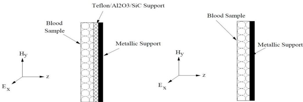
**Figure 1: Schematic Illustration of a Human Blood Sample Placed on Composite Supports Exposed to Plane Electromagnetic Waves.**
