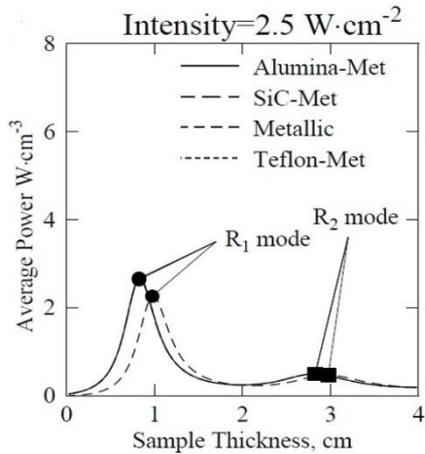
**Figure 2: Average Power vs Sample Thickness Diagram for Blood Samples Placed on Composite and/or Metallic Supports Exposed to Microwaves.**
