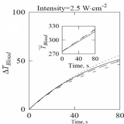
**Figure 5: Average Temperature and Temperature Difference vs Time Profiles for Blood Samples Placed on Teflon-Metallic, Alumina-Metallic, SiC-Metallic, Metallic Supports exposed to Microwaves During R1 Mode.**
