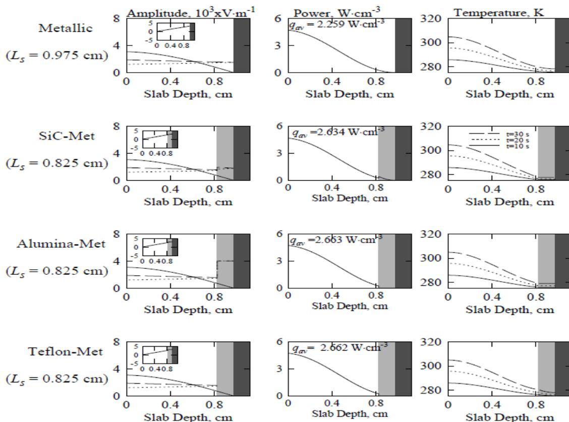
**Figure 3: Spatial Distributions of Amplitudes of Electric Field, Power and Temperature for Blood Samples Placed on Metallic, SiC-Metallic, Alumina-Metallic and Teflon-Metallic Supports during R1 Mode at support thickness 1.5 mm and intensity 2.5Wcm<sup>-2</sup>**
