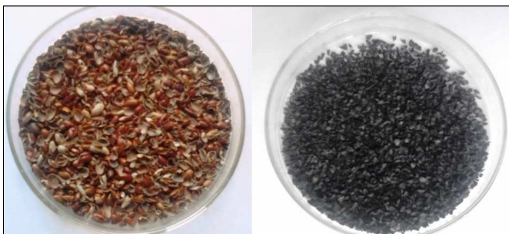
Figure 1 – Cajanus cajan seed husk converted to activated carbon
