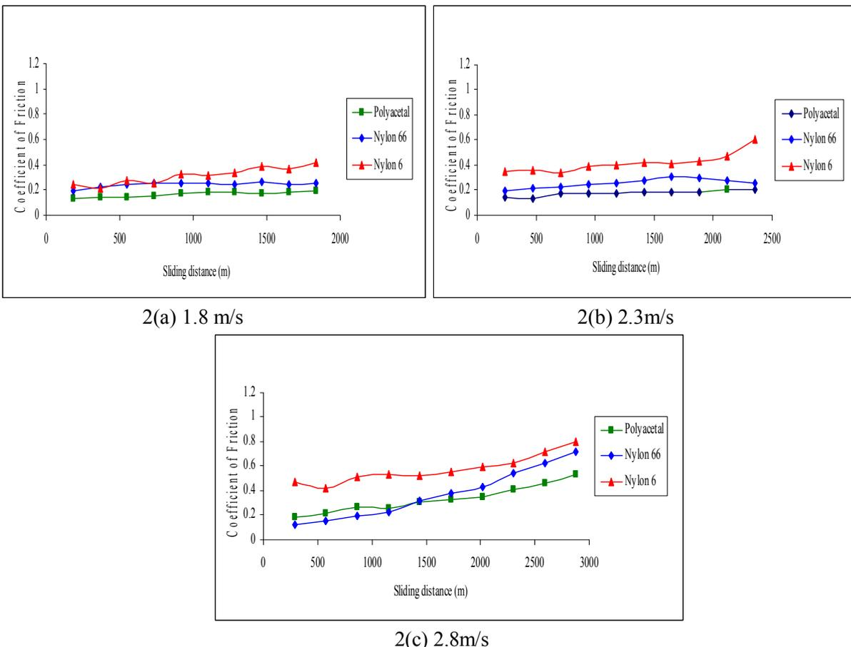
**Figures 2(a)-(c): Coefficient of friction versus sliding distance for three different sliding velocities at constant load of 60N**
