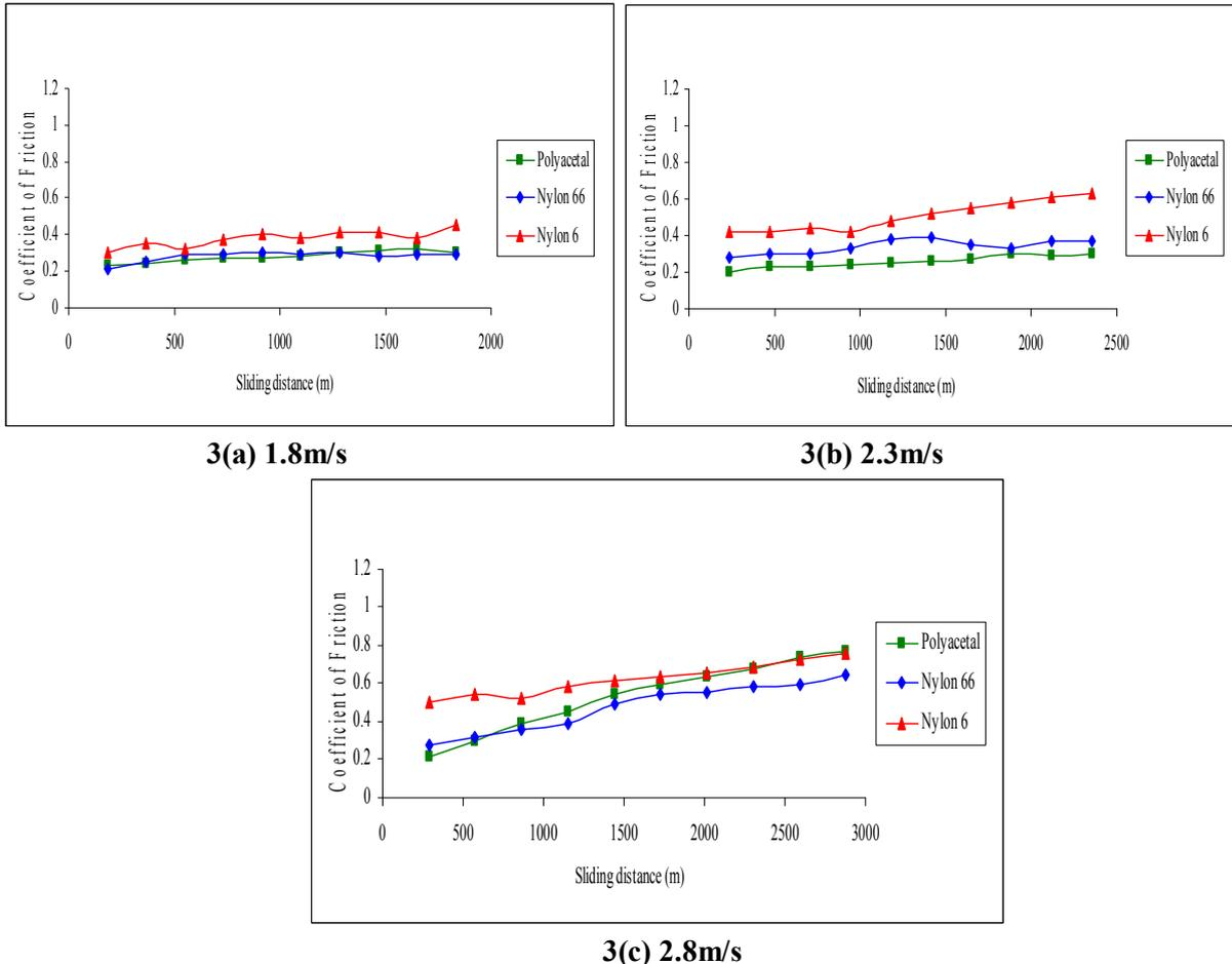
**Figures 3(a)-(c): Coefficient of friction versus sliding distance for three different sliding velocities at constant load of 80N**
