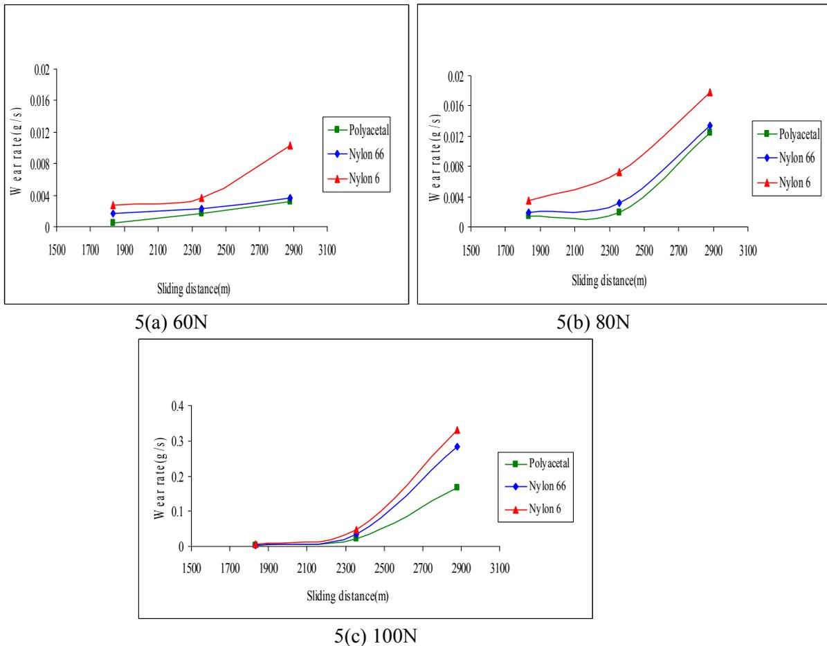
Figures 5(a)-(c): Wear rate versus sliding distance for three different loads.
