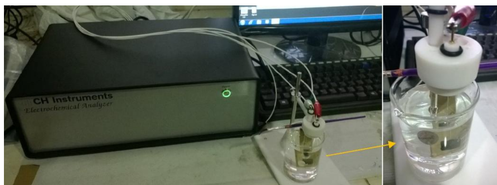
Fig.2 Experimental Setup showing the samples subjected to Potentiostat corrosion studies
