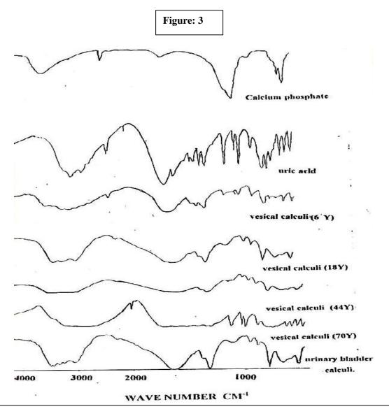
Infrared spectrum of Calcium Phosphate, uric acid, vesical calculi (6Y. 18Y, 44Y and 70 Y) and urinary bladder calculi
