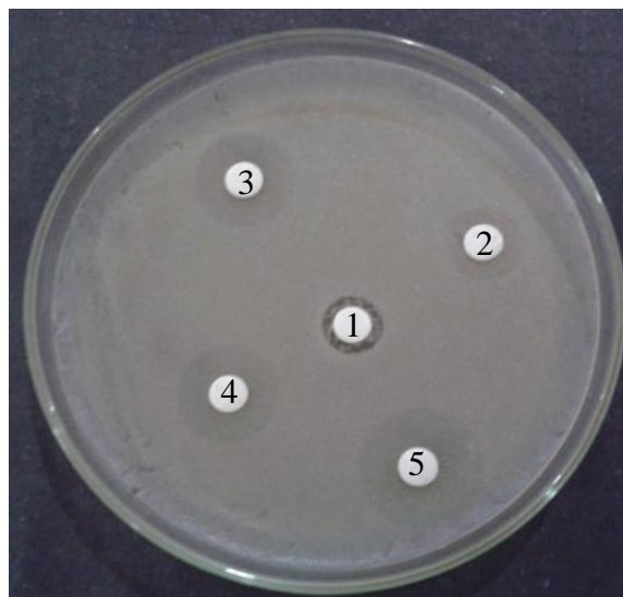
Fig. 3 Antimicrobial susceptibility of pyocyanin pigment toward E. coli by Disc diffusion method 1 – control; 2 – 5 ug/ml; 3 – 10 ug/ml; 4 – 15ug/ml; 5 – 20ug/ml
