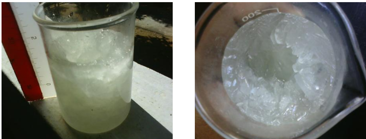
Fig. 3: Zinc Oxide crystal grown from solution (a) side view (b) top view
