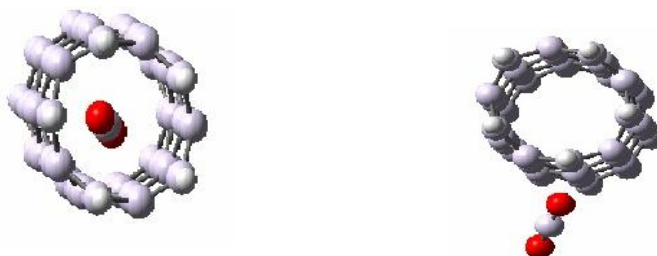
Figure.2. (D 1 ) and (D 2 ) adsorption configurations of dioxide carbon molecules
