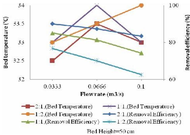
Fig 1 (a): Effect of Temperature on biofilter for the bed height of 50 cm
