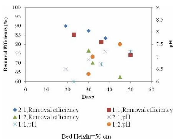
Fig 3(a): Effect of pH on Biofilter for the bed height of 50 cm
