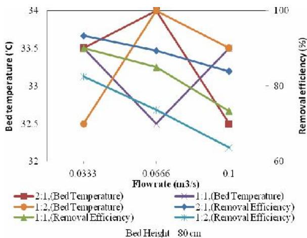
Fig 1(c): Effect of temperature on biofilter for the bed height of 80 cm
