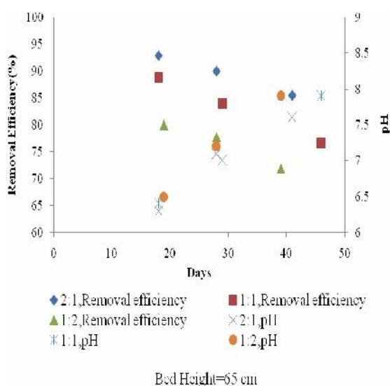
Fig 3(b) : Effect of pH on Biofilter for the bed height of 65cm
