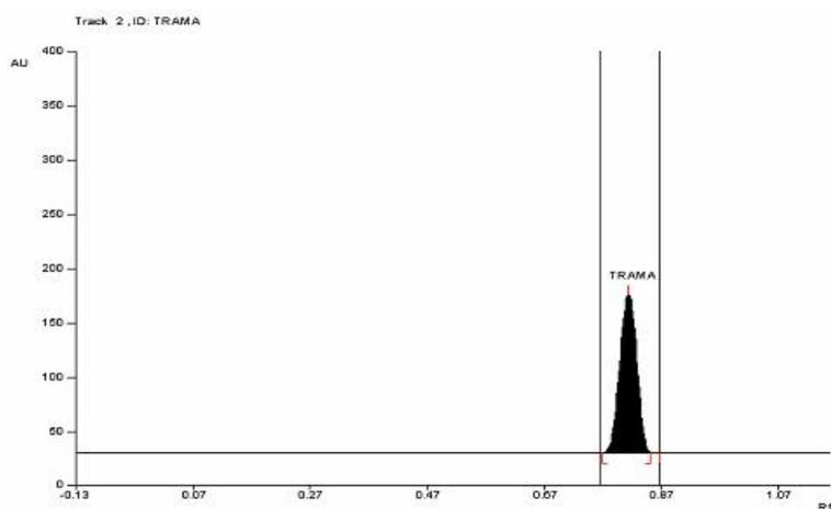
**FIG 4. HPTLC CHROMATOGRAM OF TRAMADOL HCL STANDARD SOLUTION**
