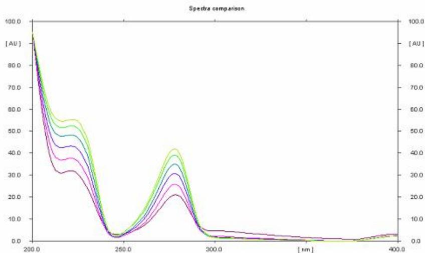
**FIG 3. UV ABSORPTION (REFLECTANCE MODE) OF THE CORRESPONDING SPOTS FOR TRAMADOL HCL**
