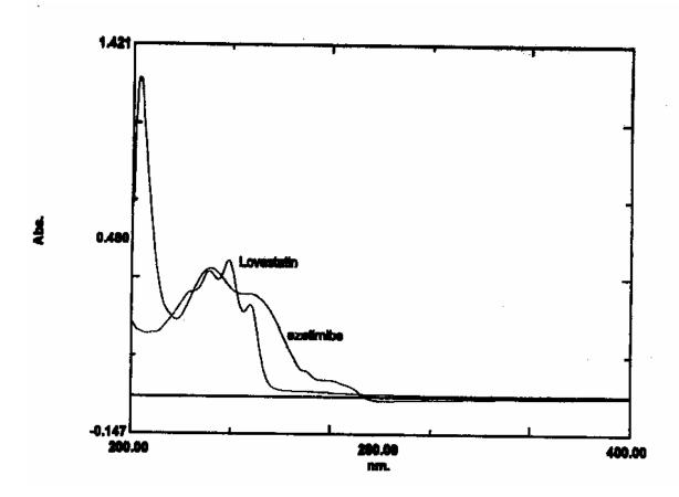
Zero order spectra of (a) ezetimibe (10  $\mu$ g/ml) and (b) lovastatin (10  $\mu$ g/ml).
