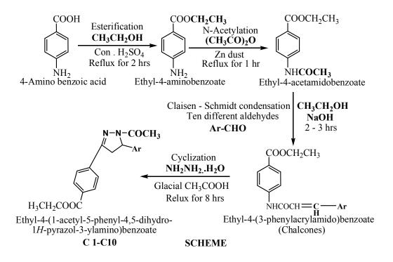
C<sub>1</sub> R – Benzaldehyde, C<sub>2</sub> R – Salicylaldehyde, C<sub>3</sub> R – p – Chloro benzaldehyde, C<sub>4</sub> R – o – Chloro benzaldehyde, C<sub>5</sub> R – o – Nitro benzaldehyde, C<sub>6</sub> R – m– Nitro benzaldehyde, C<sub>7</sub> R – p – Hydroxyl benzaldehyde, C<sub>8</sub> R – p – Dimethylaminobenzaldehyde, C<sub>9</sub> R – 3, 4, 5 – Trimethoxy benzaldehyde, C<sub>10</sub> R – Anisaldehyde.
