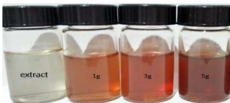
Figure 1. Change of color synthesis of silver nanoparticles. Note: Extract (1 g goroho banana peel), 1 g (sample A), 3 g (sample B) and 5 g sample C
