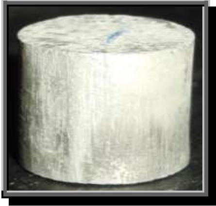
Fig. 4b Upset test preform before deformation.
