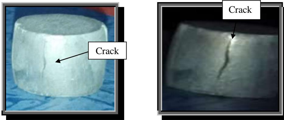
Fig. 5 Photographs showing upset test preform of after deformation test.
