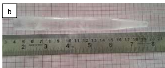
Fig.1 b) Praseodymium doped KDP <101> crystal grown by SR method
