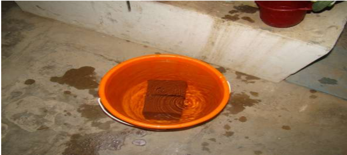
Figure 2: Brick immersed in water for 24 hours
