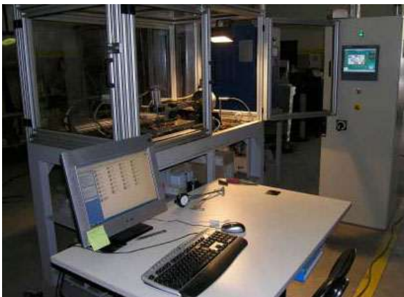
Figure 1. Honing test machine.
