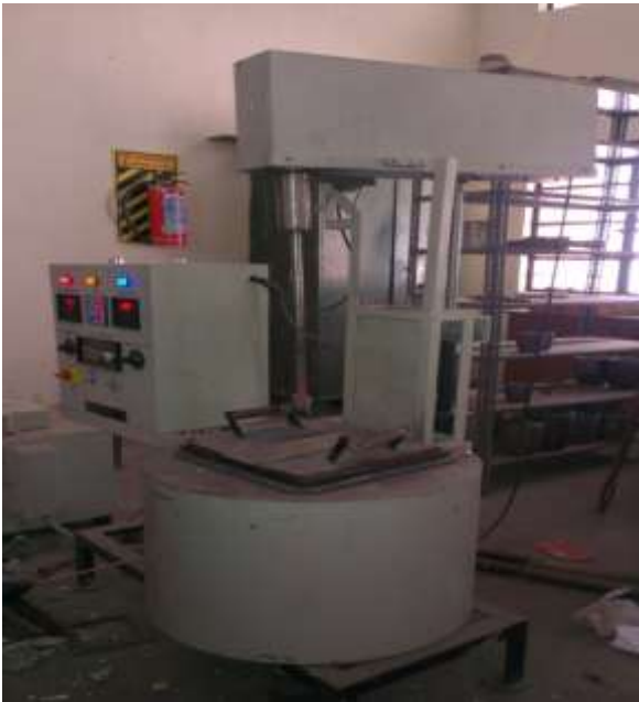
Figure 3.3.2 Aluminium stir casting setup
