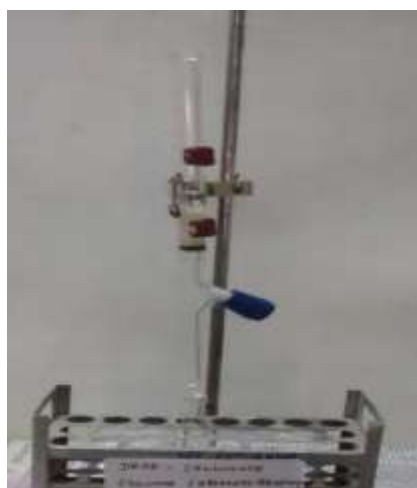
Figure 5: DEAE-Cellulose column chromatography
