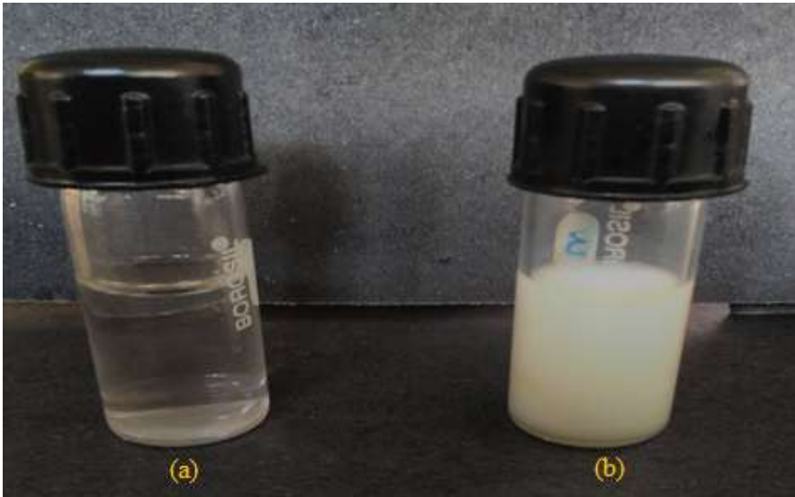
Figure.1: (a) zinc sulfate heptahydrate and urea mixture solution, (b) After addition of sodium hydroxide, formation of ZnO nanoparticle.
