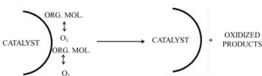
Fig. 10 Reaction mechanism for metal oxides as a catalyst in ozonation process[4]
