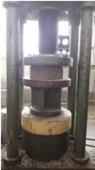
Fig.6.1 Testing of paver block
