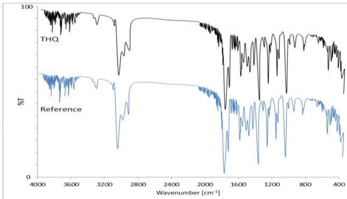
**Figure -8:** FT-IR spectra of Thymoquinone showing characteristics band and stretching.
