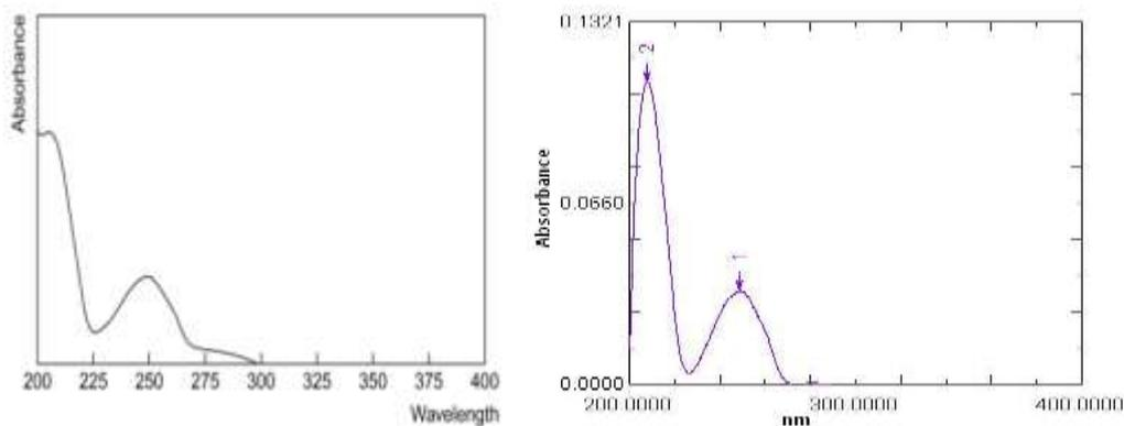
**Figure-5: Comparison of UV-spectra of Thymoquinone in methanol ( $\lambda_{\max}$  – 254 nm) with reference**
