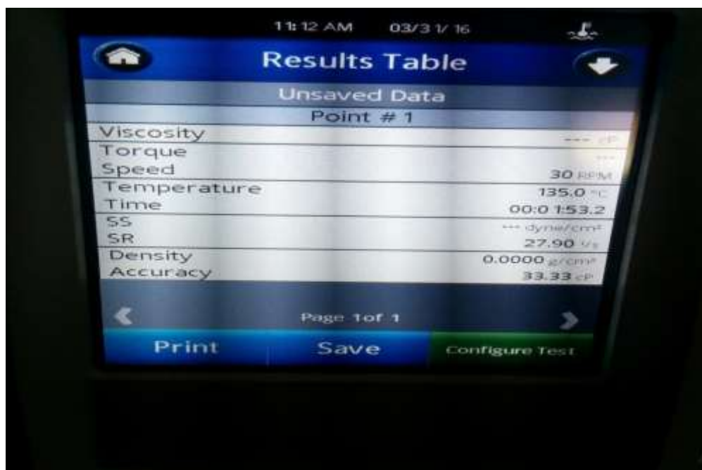
Figure 4 – Digital test result representation of viscosity.
