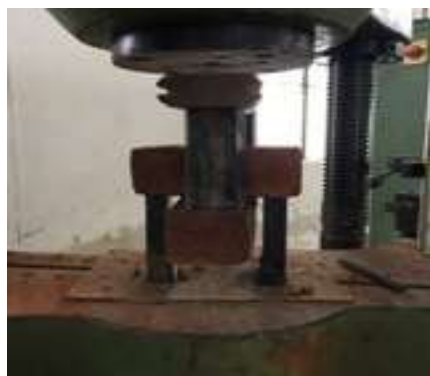
Fig 1 Testing of brick couplets
