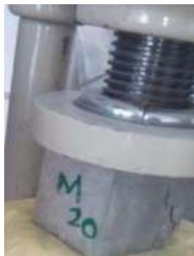
Figure 1: Test setup of cube in compression Figure 2: Crack formed in the cube testing machine
