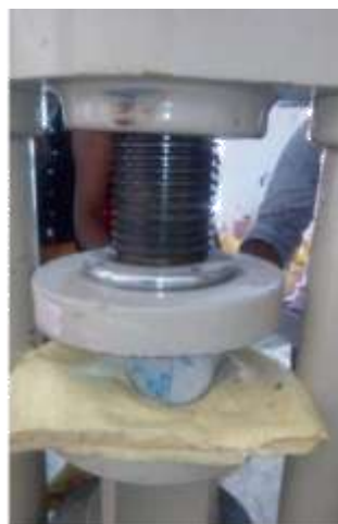
Figure 3 & 4: Test setup of cylinder for split tensile strength test & Crack formed in the cylinder.
