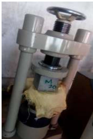
Figure 1: Test setup of cube in compression Figure 2: Crack formed in the cube testing machine
