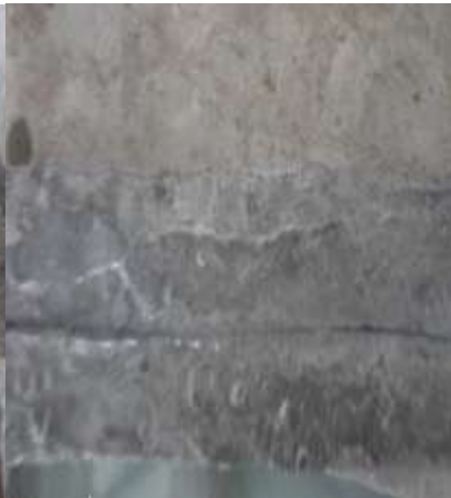
fig 5.4 self healing after 60 days curing bacterial concrete
