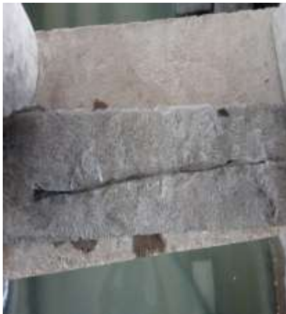
fig 5.3 self healing after 60 days curing control concrete
